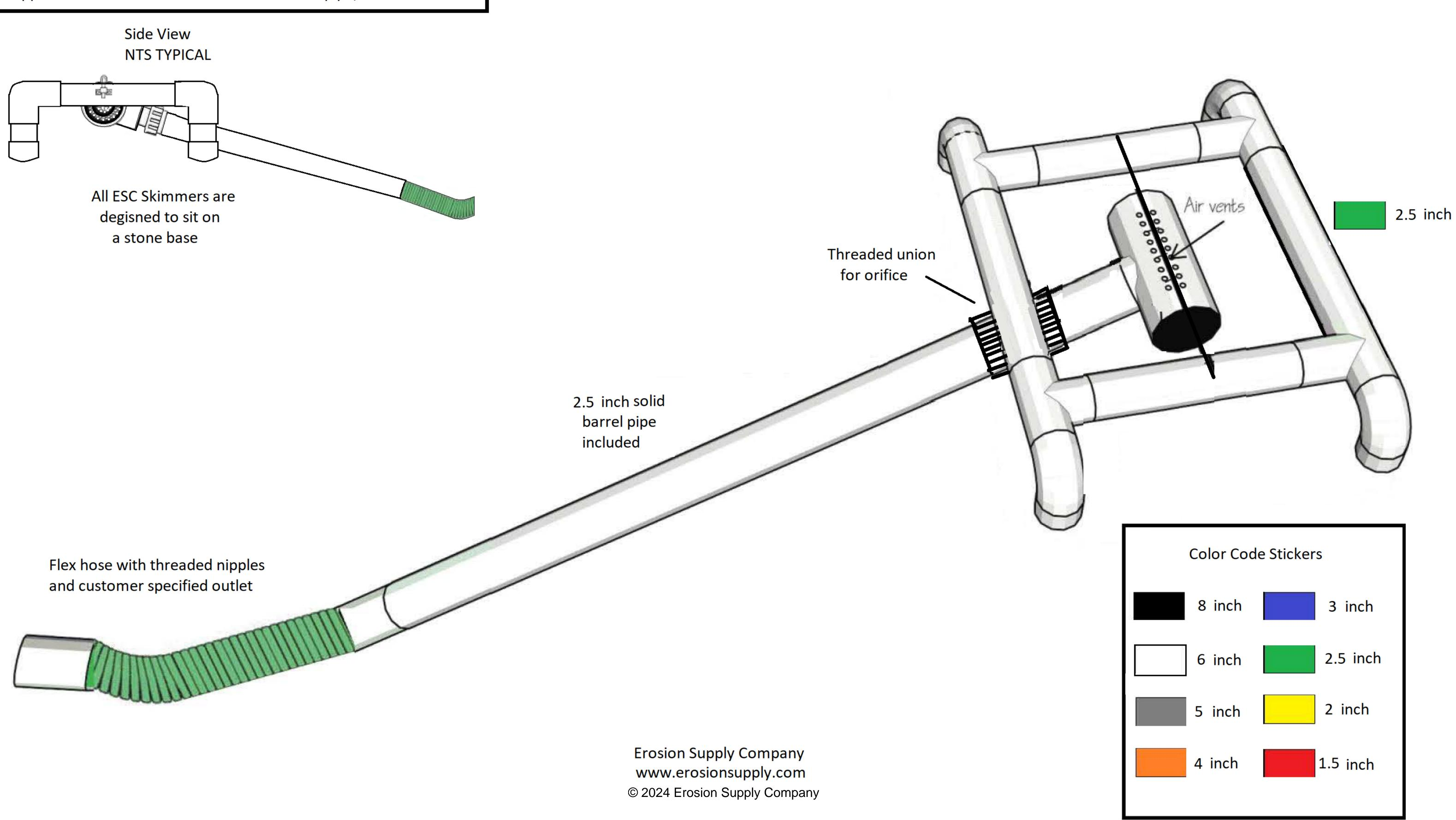
2.5 inch ESC Skimmer / Sediment Pond Surface Drain
